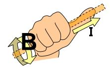
Point your fingers in the direction of the magnetic field (B) and your thumb in the direction of the current (I). The palm of your hand will push in the direction of force (F).
